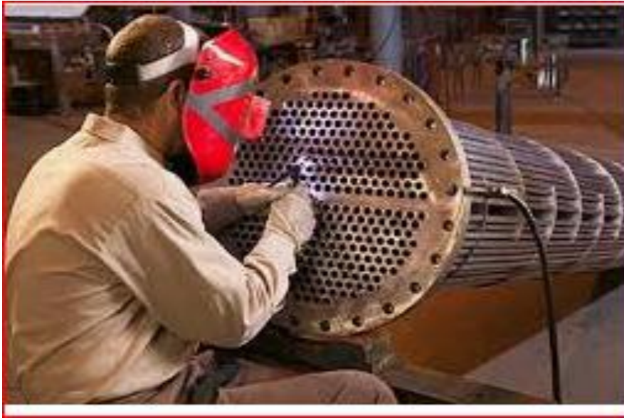
Fig.27. Heat exchanger pipe maintenance
